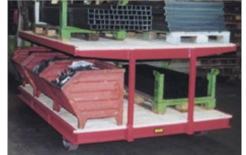
Additional loading surface in the form of a plug-in level
