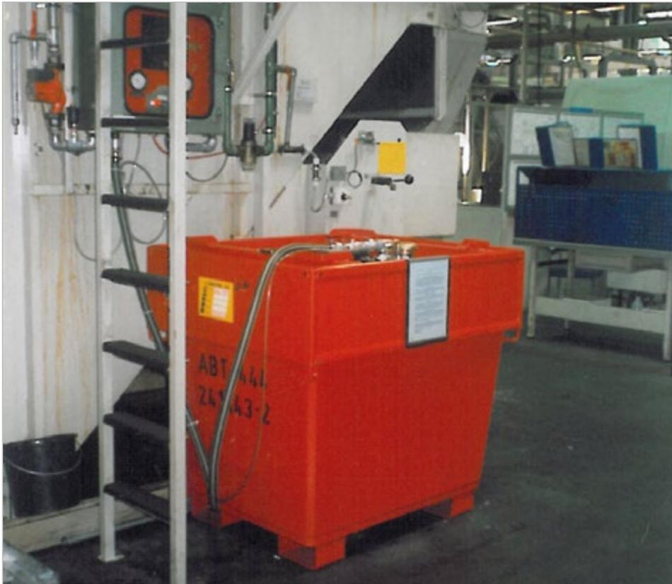
Supply and disposal of flammable liquids with a flash point > 55° C.
