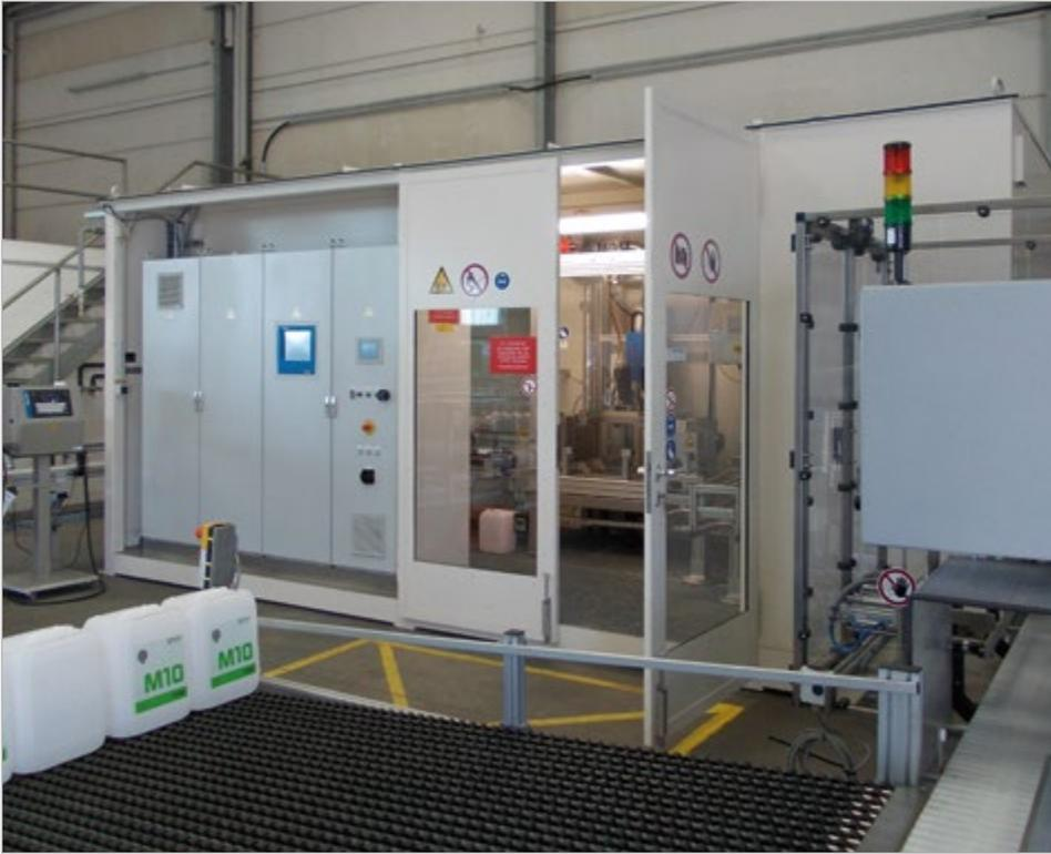
**Insulated container for indoors or outdoors - storage space or a work place for decanting/siphoning**
