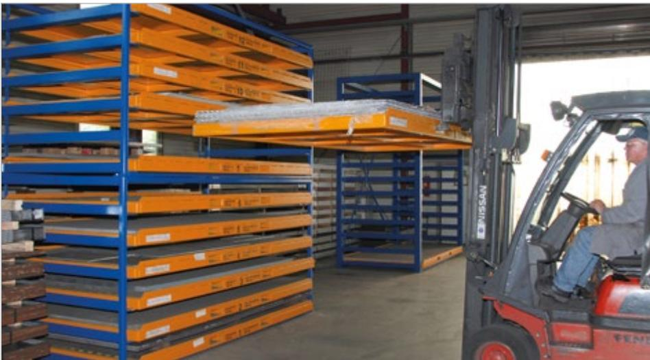
**Space-saving, clear-cut storage unit for steel sheets or other materials in plate format**
