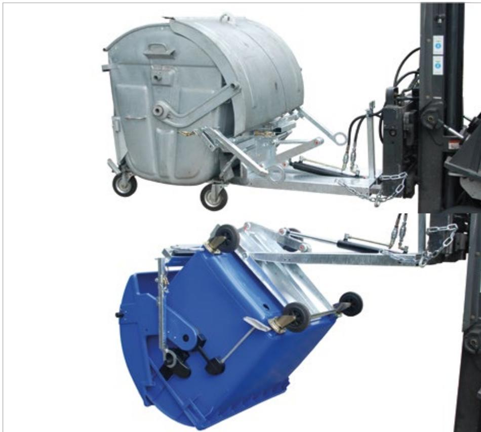
The KM is an indispensable aid for transporting, emptying and cleaning large volume wheelie bins (1100 litres with 4 wheels) and manufactured to DIN EN 840-3
