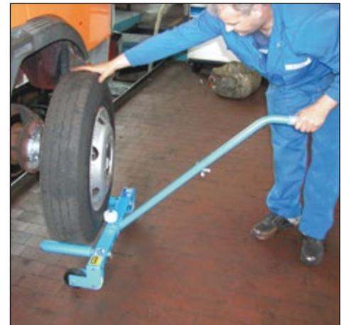
Easy tyre fitting for trucks, busses and forklift trucks
