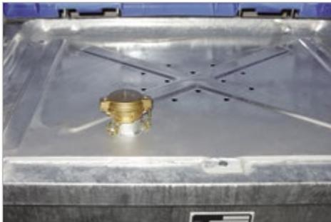
Filling tray and 2" tank truck coupling
