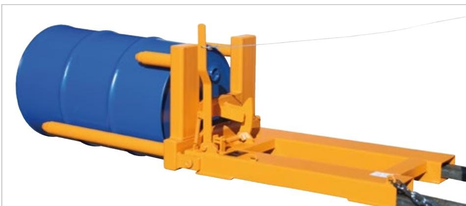
To upright 200 litre steel bung hole drums and rolling hoop drums from a horizontal position or to store them lying down
