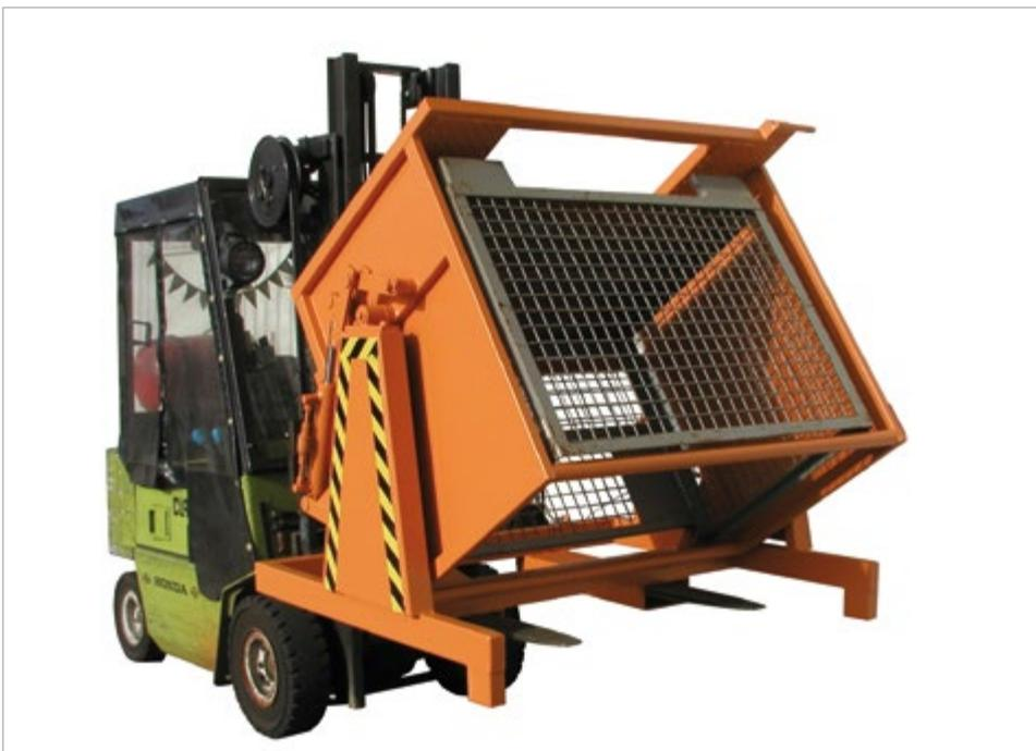
Type KGM with adjustable dumping brake
