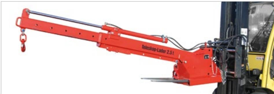
Extended hydraulically (Type KTH)
